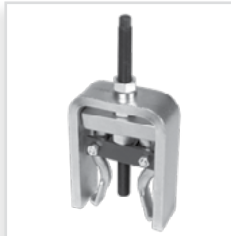
T3916 Pilot Bearing Jaw Spread 1" To 1.5" I.D. Reach .75" Applicable For Use On Most Models with Engine In Chassis
