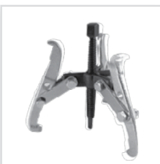
T3906 2 Ton Capacity 2 or 3 Jaw Gear Puller Maximum Reach 3.375" Maximum Spread 4" Adjustable and Reversible Jaws
